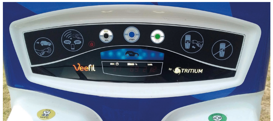
Figure 1: A Tritium DC charger display—note the 80% or maximum button.
