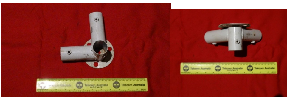
Corner wall pole to ground bar connectors (Part No. 6).
